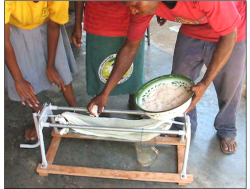
Placing the grated coconut into the squeezing bag
